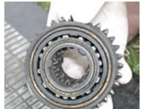
5-2-5. This picture shows one of the dogs located correctly in its slot.
