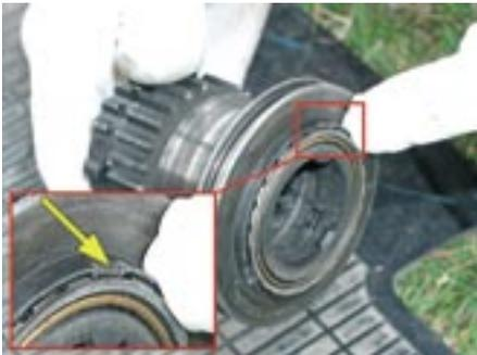
5-2-2. The ring for the second and third gear selector fork was staked onto the synchro hub when the gearbox was built (inset, arrowed). The problem is that the three stakings may not hold, especially on the later gearboxes.
