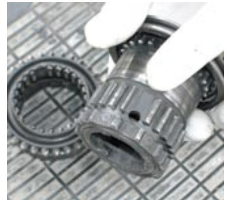
5-2-4. This internal ring has three dogs on it which slide in three slots on the second and third synchro hub. The dogs can come free of the slots, and the ring on which they are located can turn so that the dogs no longer line up with the slots. You then have the job of realigning the dogs with the slots before you can get the ring back on the synchro hub. (In other words, before you can push the first gear synchro hub onto the second and third gear synchro hub.)
