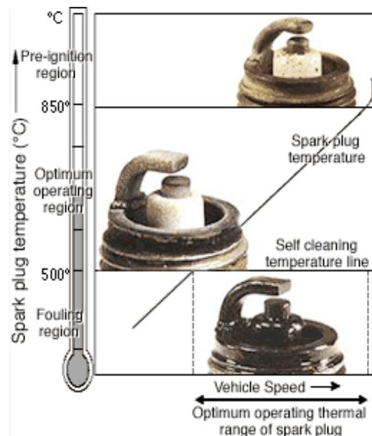
The firing end appearance also depends on the spark plug tip temperature. There are three basic diagnostic criteria for spark plugs: good, fouled and overheated. The borderline between the fouling and optimum operating regions (500°C) is called the spark plug self-cleaning temperature. The temperature at this point is where the accumulated carbon and combustion deposits are burned off.
